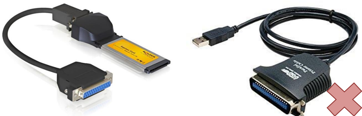
Figure 6: Parallel port express card (left; correct) and parallel port USB adapter (right; incorrect).
