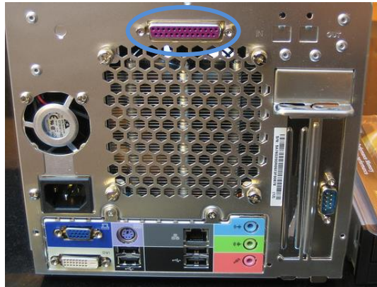
Figure 5: Parallel port of a computer, located on the back of the chassis. Note: The Parallel port is not always colored purple.
