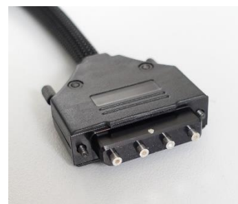
The laser fiber receptacle is equipped with a sensor which interrupts the laser radiation whenever the laser fiber plug is removed from the receptacle. This is a safety feature to avoid a freely propagating laser beam to be emitted by the instrument and to make sure that laser radiation is applied to the tissue only through the proper optical fiber bundles. The sensor is activated by a small magnet that is situated near the front edge of the laser fiber connector (see picture). Fig. 12: Difference between the connections used for laser and detector fiberoptics. Left: Comparison of plug for laser (bottom) and detector(top) cable. Center: Receptacle for laser fiber. Right: Receptacle for detector fiber.
