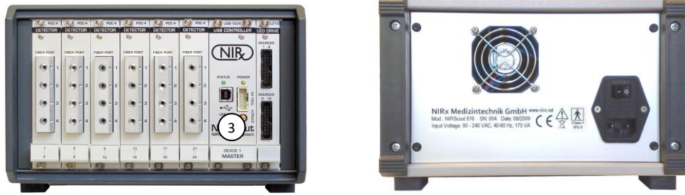
Fig. 2: (a) Front view of the NIRScout imaging system. (1) Quad-channel detection cards QDC-10; (2) USB controller card USB-1618 with Trigger input (3); (4) Led driver card LED-16. (b) Rear View showing AC power inlet and power main On/Off switch (1).
